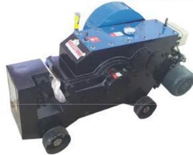
Bar Cutting Machine Model: GQ-40, Capacity: 6-32 mm Cutting Frequency: 32 r/min Motor: 3 KW, Volt: 415, Weight: 330 Kg.
