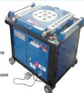
Bar Bending Machine Model: GW-42A Capacity: 6-32 mm, Speed: 5-15 r/min Motor: 3 KW – 3 Phase RPM: 1440, Volt: 380, Weight: 280 kg.
